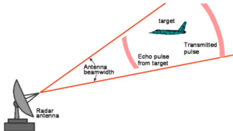
Gambar 7. Prinsip pengoperasian radar
